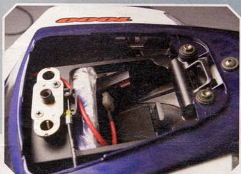
The SpeedoHealer mounts cleanly and compactly out of the way under the rear passenger seat, and it works.
